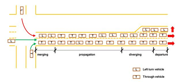
Figure 4-2 Link spillback blockage at the merging zone
