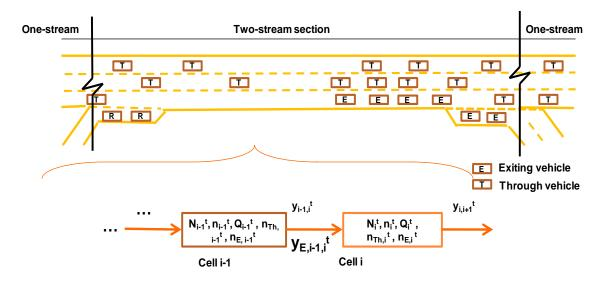
Figure 5-4 Modeling of the two-stream interaction in a Type-A segment by cell
