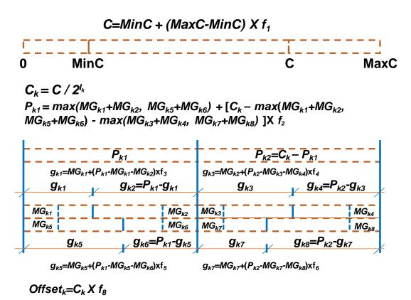
Figure 4-11 An enhanced fraction-based decoding scheme for signal design
