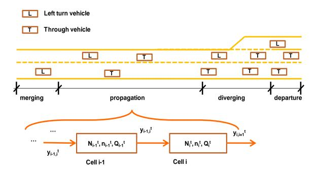
Figure 4-4 The propagation zone represented with ordinary cells
