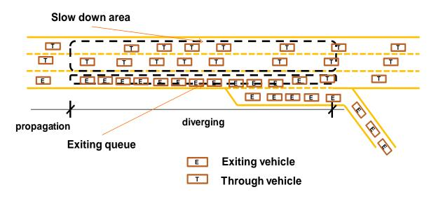
Figure 5-7 Exiting-queue effect in a diverging zone
