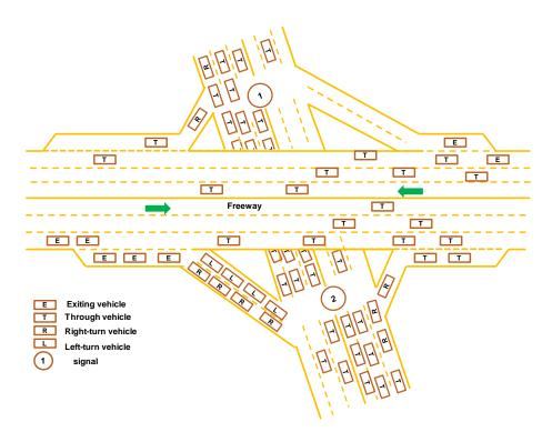
Figure 5-1 Graphical illustration of a signalized interchange
