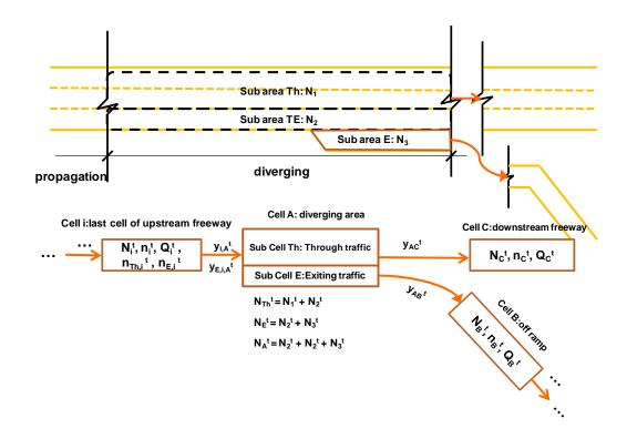
Figure 5-8 Graphical illustration of the modeling concept for the diverging zone
