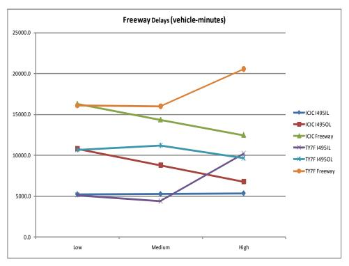
Figure 6-4 Comparison freeway delay by segment
