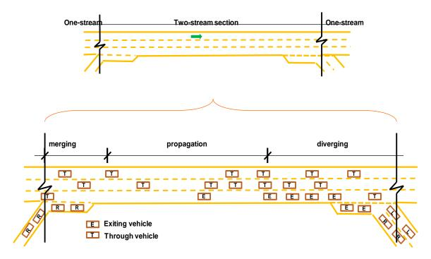
Figure 5-5 Type-A segment traffic dynamics
