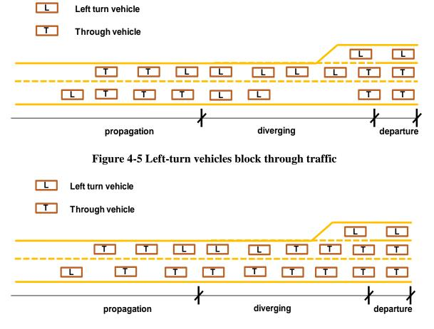
Figure 4-6 Through vehicles block left-turn traffic
