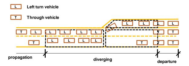
Figure 4-9 An illustration of left-turn queue blocking through traffic
