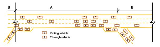
\*Type-A segment: vehicles can go either to the downstream mainline segment or off-ramps.
