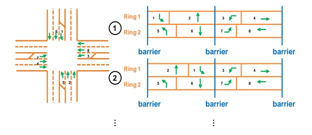
Figure 4-10 NEMA eight-phase signal timing structure
