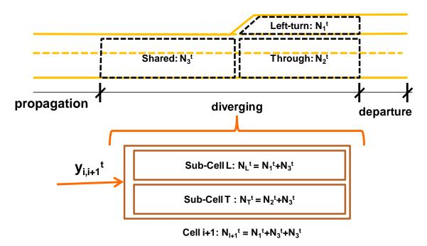
Figure 4-8 The sub-cell representation of a diverging signalized cell
