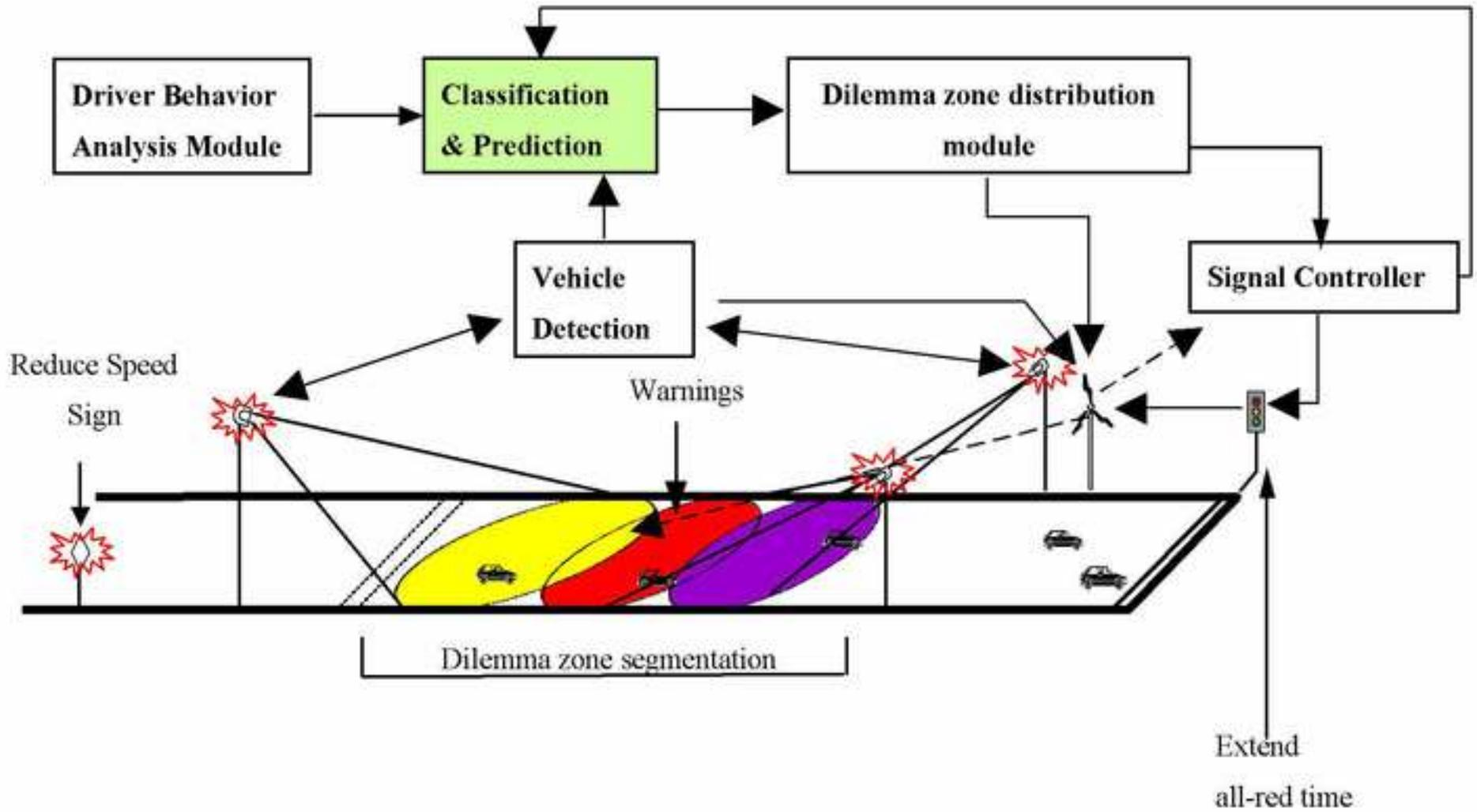
Fig. 5. ITS-based dilemma zone protection system design
