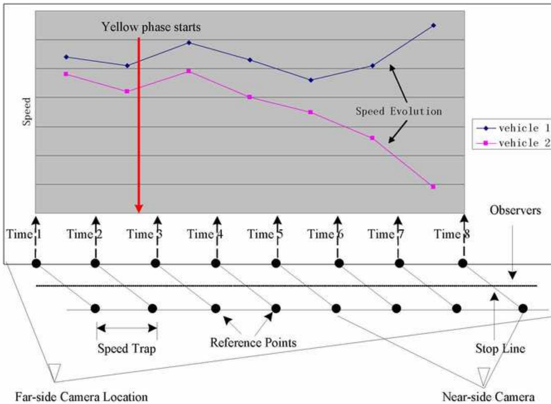
**Fig. 1.** A graphic illustration of the video-based data collection system – design and components
