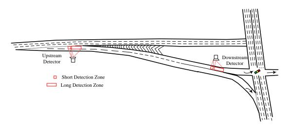
Figure 1 Location of dual-zone detectors on the target off-ramp
