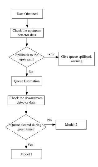
Figure 6 Flowchart of the entire queue estimation process
