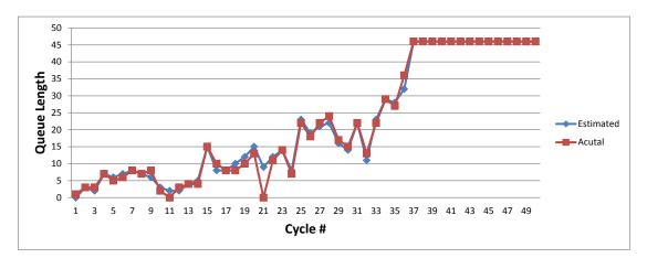
Figure 10(A) The comparison between estimated queue and actual queue
