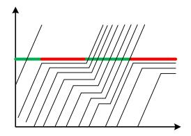
Figure 5(B) Queuing vehicles cannot be fully discharged during the green phase
