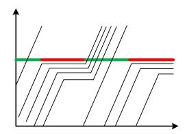
Figure 5(A) Queuing vehicles can be fully discharged during the green phase
