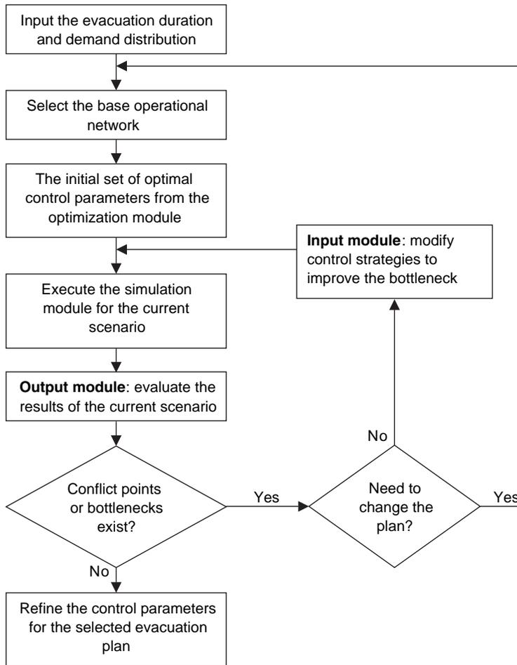
FIGURE 5 Operational flowchart for planning hurricane evacuation.
