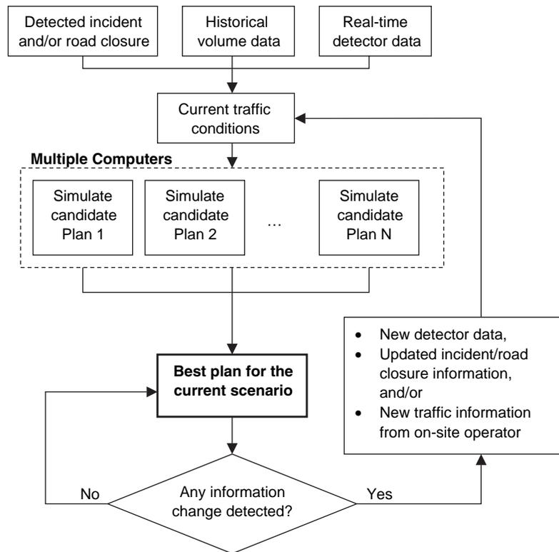
FIGURE 9 Operational procedures for real-time evacuation operation.
