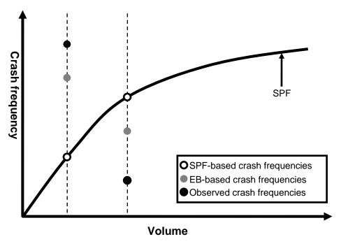
Figure II.1 EB-based, SPF-based and observed crash frequencies
