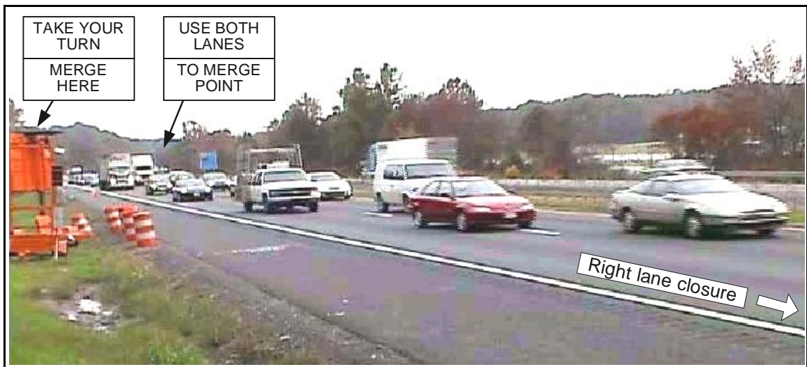
Figure 4.1.1 Merging behavior prior to the merge point under the congested traffic condition (e.g., SLM)
