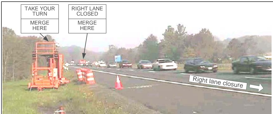
Figure 4.1.2 Merging behavior prior to the merge point under the non-congested traffic condition (e.g., SEM)
