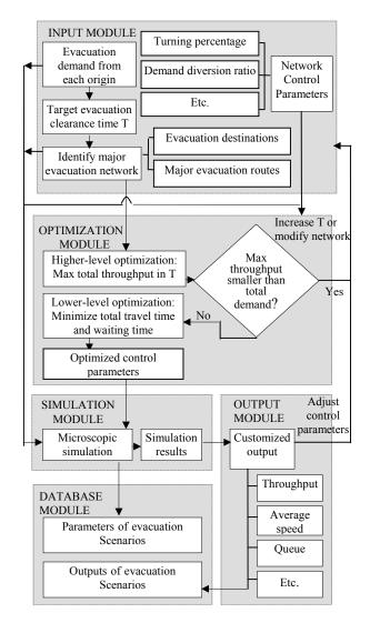
Fig. 2. Framework of the integrated evacuation system
