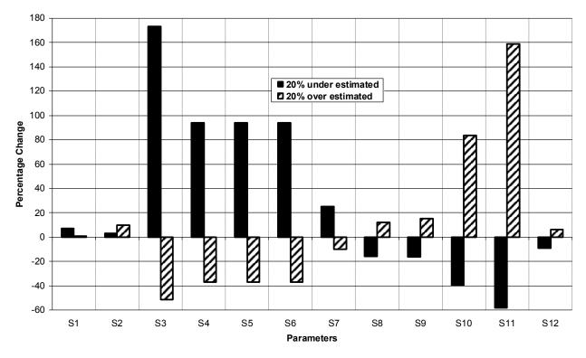
Figure 6. Percentage change of total toll collected for the system optimal solutions with 20% inaccuracy in input parameters
