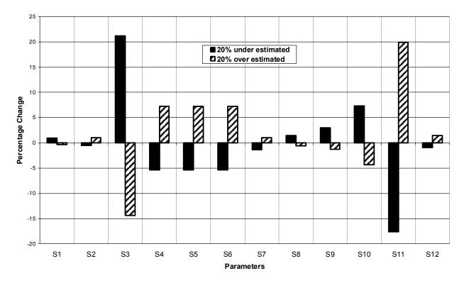
Figure 4. Percentage change of demand for the system optimal solutions with 20% inaccuracy in input parameters
