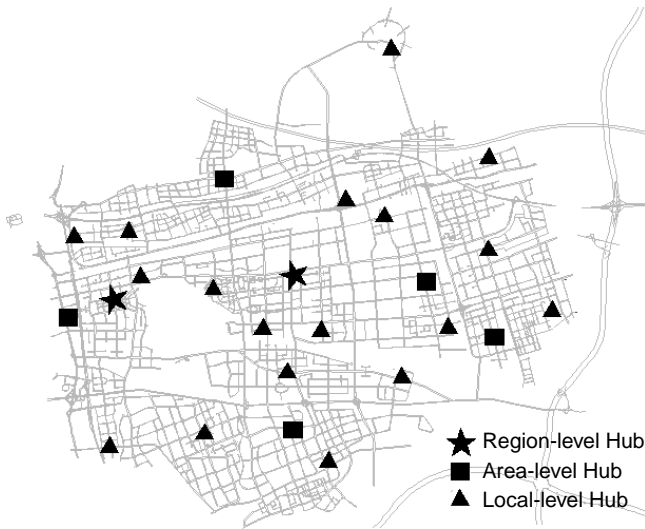
FIGURE 6 Optimal locations of the transit hubs from the model.
