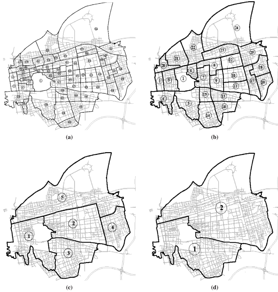
FIGURE 5 Study network layout: (a) 58 TAZs in the study network, (b) 25 clusters in study network, (c) five service zones for five area-level hubs, and (d) two service zones for two region-level hubs.
