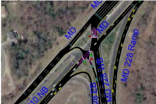
Figure 5. CORSIM Simulation of the CFI, MD 210 @ MD 228 comparing the conventional T-intersection with the CFI T-intersection.
