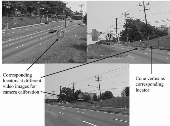
Fig. 5. Camera calibration
