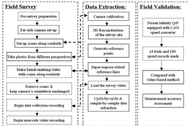
Fig. 3. Operational procedures of the video-based measuring system
