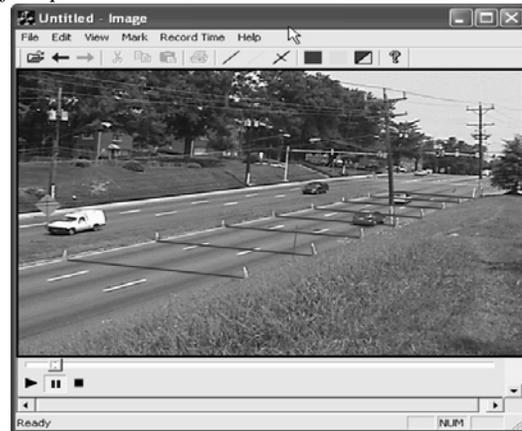
Fig. 6a. Benchmarking with cones or reference points
