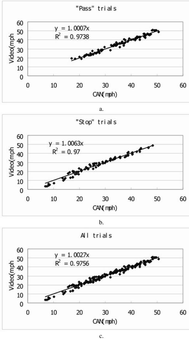
Fig. 7. Speed measurements by video versus the CAN converter
