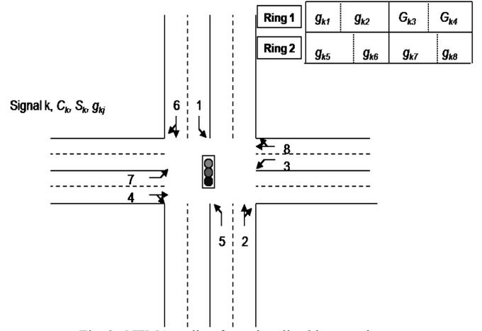
Fig. 3. NEMA coding for a signalized intersection
