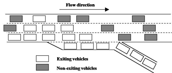
Fig. 1. Lateral spreading of an exiting queue upstream of an off-ramp.
