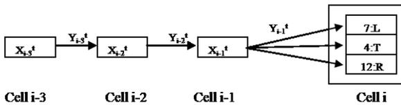
Fig. 5. Diverging cell connection for approaching road segment
