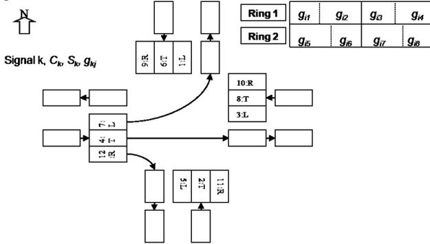
Fig. 4 Deployment of a four-leg intersection
