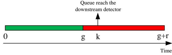
**Figure 8 Time slots within the target signal cycle**
