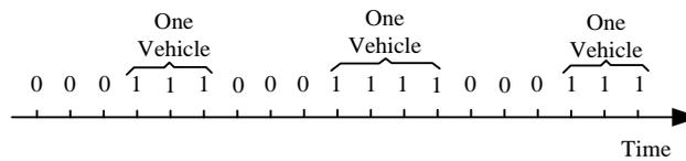
**Figure 3(A) The recording of number of passing vehicles by the short detection zone**
