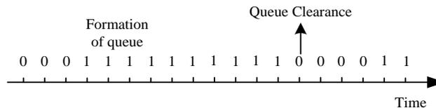
**Figure 3(B) The detection of queue formation and clearance by the long detection zone**
