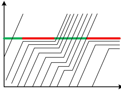
**Figure 5(B) Queuing vehicles cannot be fully discharged during the green phase**
