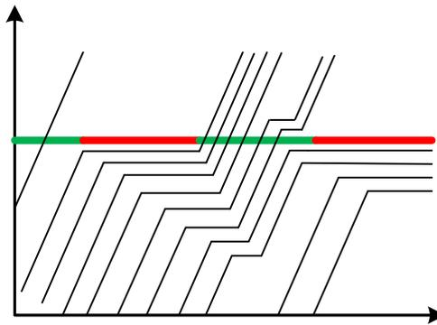
**Figure 5(C) Queue spillover at downstream link may affect the discharging process**
