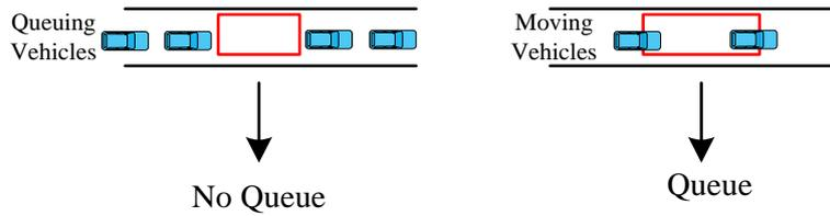
**Figure 4(B) Identification errors caused by long detection zone**
