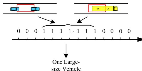
**Figure 4(A) Identification errors caused by short detection zone**
