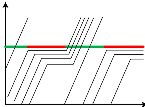
**Figure 5(A) Queuing vehicles can be fully discharged during the green phase**
