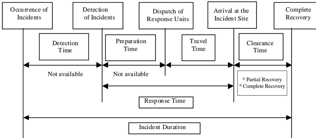
**Figure 4. A Graphical Illustration of Technical Terms Associated with an Incident Operation** (Source: *Performance Evaluation of CHART. Final Report 1997*)
