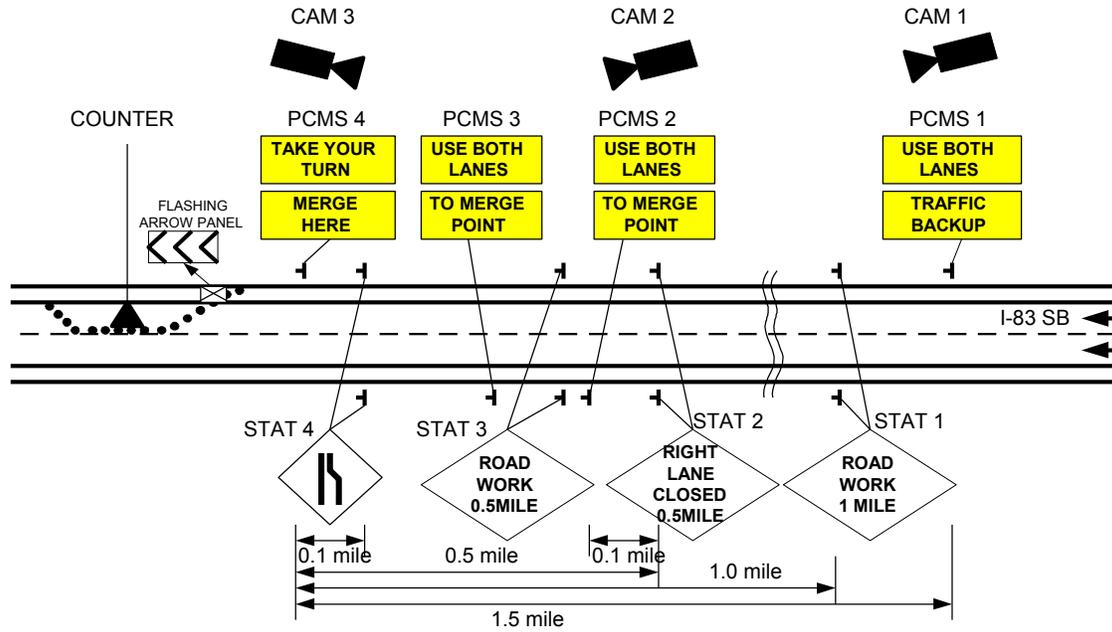
FIGURE 1 Configuration of the DLM system and data collection.
