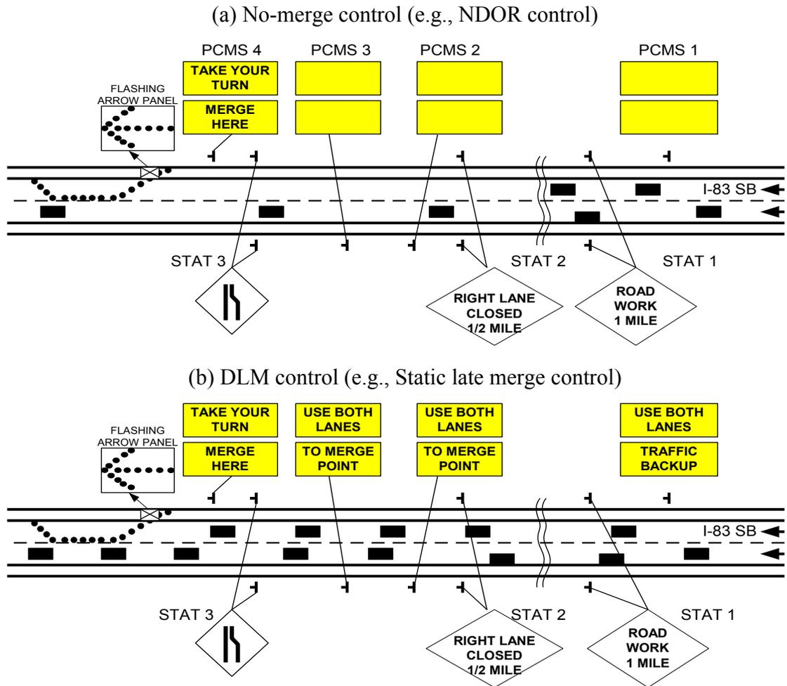
**FIGURE 2** Traffic conditions and merging messages under the No-merge and DLM controls.
