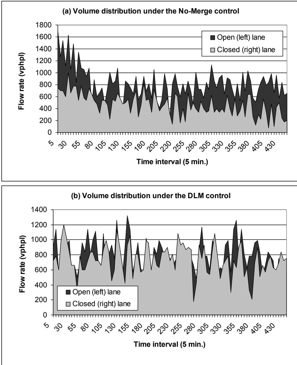
**FIGURE 5** Volume distribution between the open (left) and closed (right) lanes at the middle point under the No-merge (a) and DLM (b) controls.
