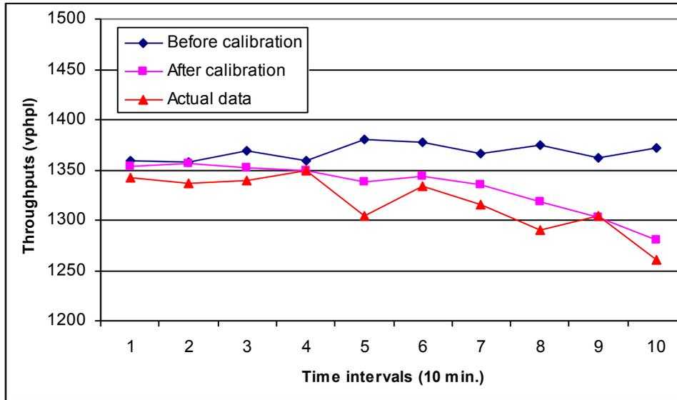
**FIGURE 4 Comparison of the work zone throughputs under the simulated work zone operations.**
